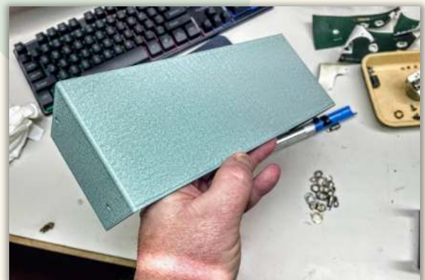
Clockwise from left: disassembly of the burned unit, checking operation; stripping the old artwork off to prepare for new artwork; repainting the box and lid with Heathkit SB-color spray paint
