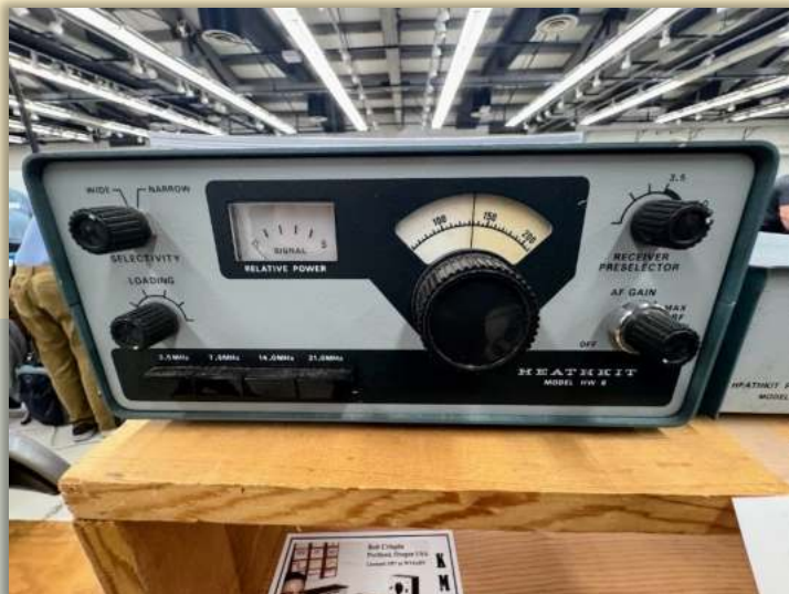
One of the icons of the QRP world: The venerable Heathkit HW-8 designed by Bob Furnau, W8NDG (SK)
