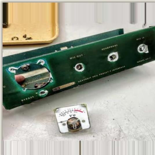
Clockwise from left: disassembly of the burned unit, checking operation; stripping the old artwork off to prepare for new artwork; repainting the box and lid with Heathkit SB-color spray paint
