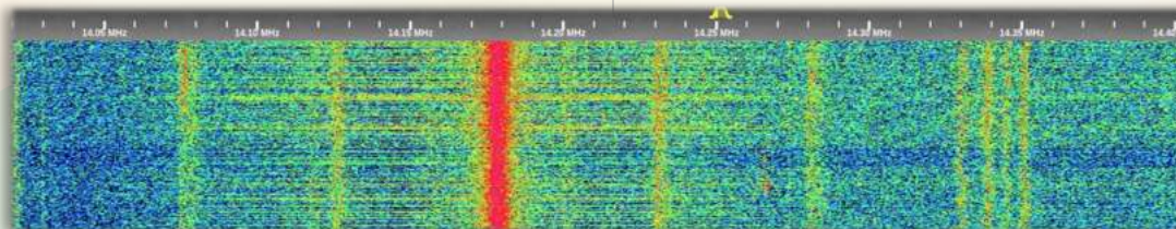
Waterfall display of a modern radio showing pretty massive RFI on the 20m band
