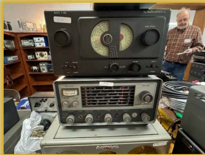
Two iconic receivers—the Hallicrafters S-38 and the SX-140—both popular and both mediocre! The S-38 was general cover, the 140 ham only
