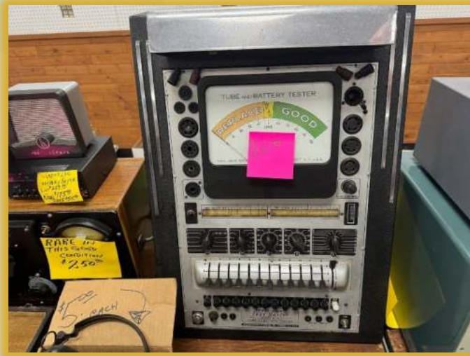
Cigarette vending machine? Pachinko? Nah... just a giant wall-mount commercial tube tester from the past called a Tube Master—once hung on a drugstore wall
