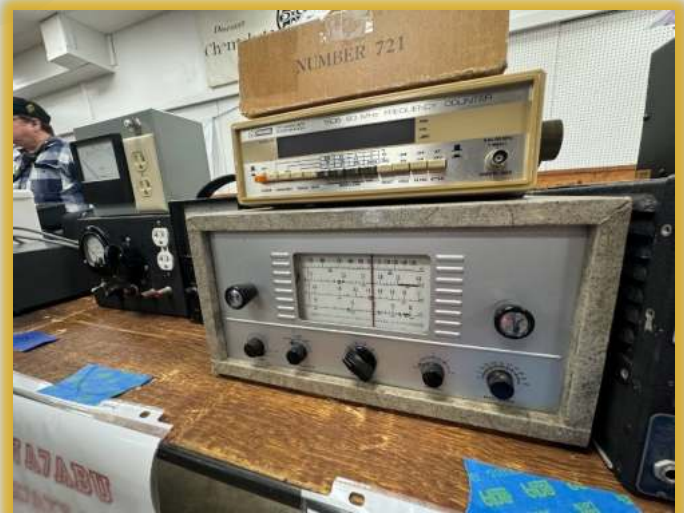
Many a Novice Ham got started with one of these receivers—the Heathkit AR-3 was the third incarnation of the design and the one that actually had the potential to make contacts vs. the prior releases of this receiver. The cabinet was not included—you had to pay extra to get it!
