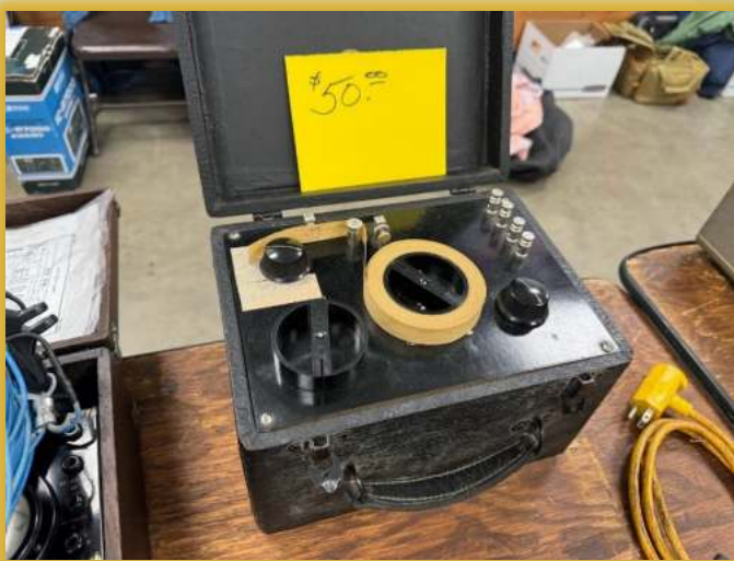
"Hams of a certain age" will immediately know this machine... an Instructograph Morse trainer using paper tapes to play code at varying speed. This is the machine used at the FCC offices in all major US cities for General and Extra testing back in the day—I took my General in Seattle from one in 1975
